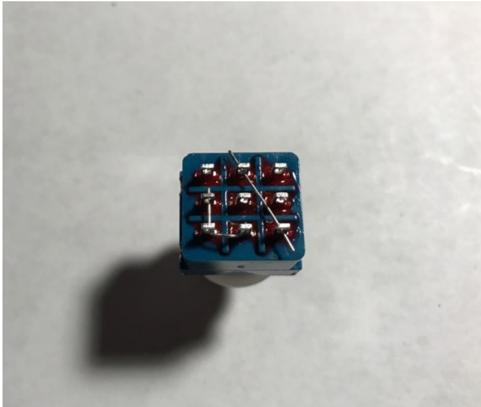
3PDT Switch Soldering Preparing switch with jumpers.
